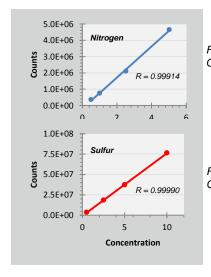
Fig.1: Calib. 0.3 – 5.0 mg N/l
